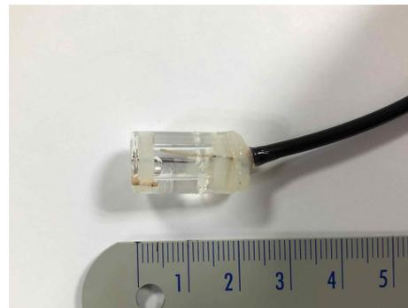
Fig. 1. Miniaturized pH electrode. (2 mm)
