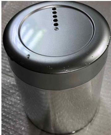
Fig. 8. Scratches on the surface.
