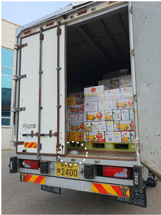
Fig. 4. Truck applied to measure the transport environment load during distribution of Seongju Korean melon and the attachment position of the field recorders.
