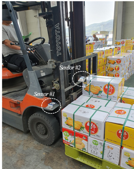
Fig. 2. Forklift truck applied to measure environmental loads for handling in APC, and the attachment position of the field recorders.
