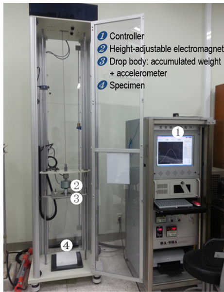
Fig. 4. Experimental apparatus for cushioning test.
