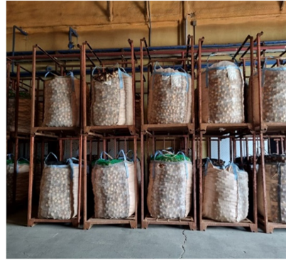
Loading of ton bag and steel pallet
