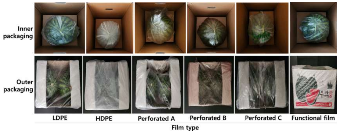
Fig. 2. Packaging treatments of seedless watermelon using six types of plastic films (LDPE, HDPE, perforated A, perforated B, perforated C, and functional prototype film with PGT+ETZ), applied as inner or outer packaging in corrugated boxes.
