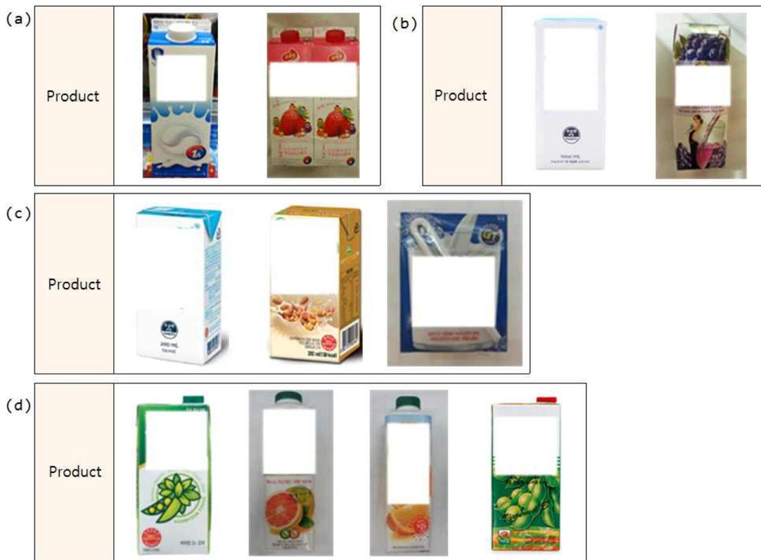
Fig. 3. Sample of cartons for liquid product that are difficult to recycle. (a) is use of synthetic resin molded product (example 1). (b) is use of aluminium lamination (example 2). (c) is use of aluminium lamination and synthetic resins straw (example 3). (d) is use of aluminium lamination and syntehtic resin molded product (example 4).
