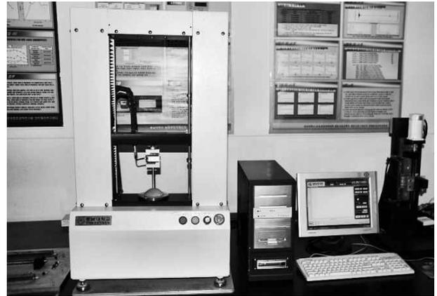
Fig. 3. Universal compression tester for fruits.
