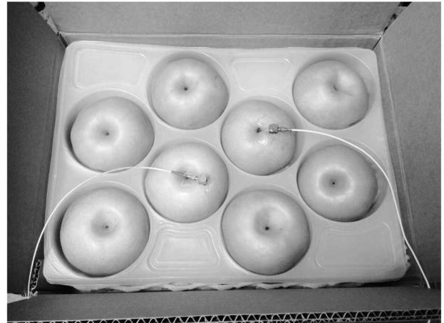
Fig. 1. Sample for parcel delivery service of pears used in sweep vibration tests.
