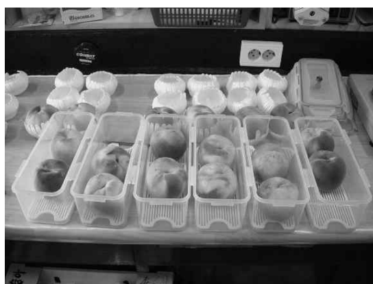
Fig. 4. Container (jar) for the ethylene gas collection of apples.
