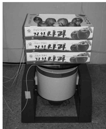
Fig. 2. Vibration test for the apples in the packaged freight.
