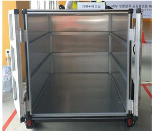
Fig. 2. Delivery box of cargo bike.
