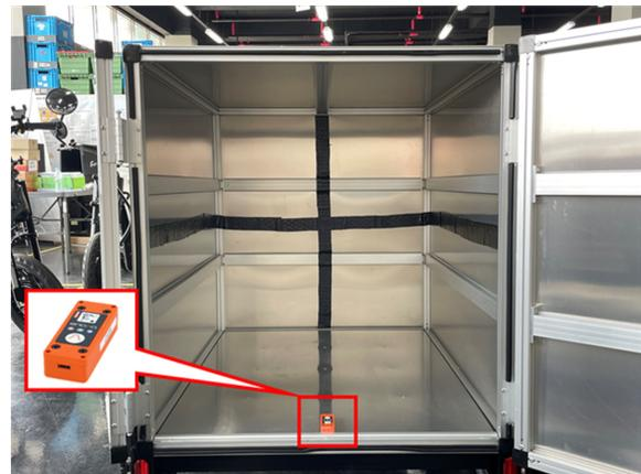
Fig. 3. Installation of the accelerometer sensor.
