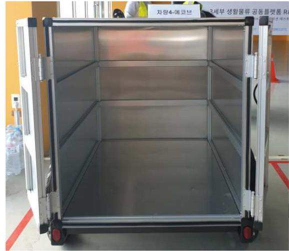
Fig. 2. Delivery box of cargo bike.
