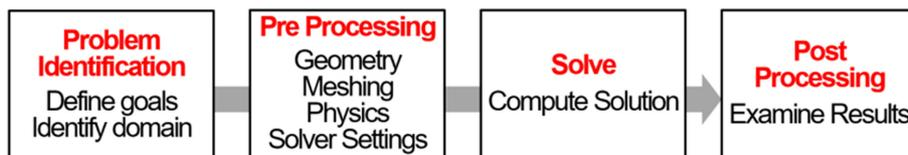
Fig. 2. CFD analysis work flow of cold storage for garlic using mech pallet container.
