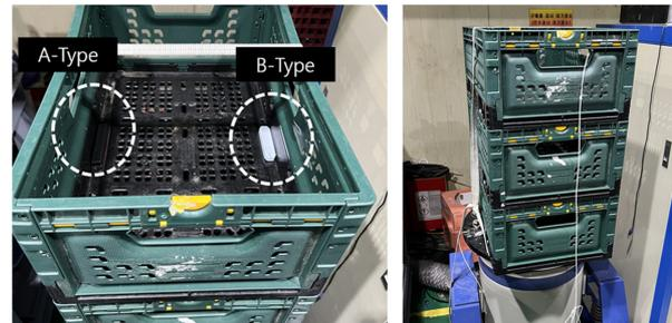
Fig. 6. Testing of type A and B integrated modules by random vibration.
